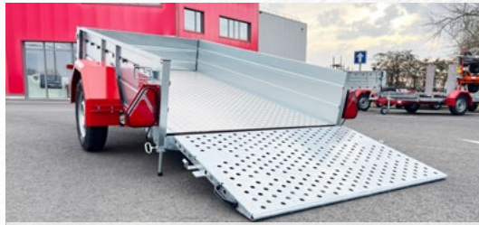
Plancher Alu, porte-pont, sign. LED (S600)
